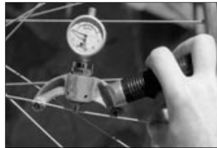
Figure 2. In use, one arm of the tensiometer is hooked under the spoke and the other is pressed down until it just touches the spoke, depressing the central plunger against spring restoring force and producing a dial reading. The tension must be read from a calibration table, as the reading is a nonlinear function of tension, spoke thickness and spoke bending stiffness.
