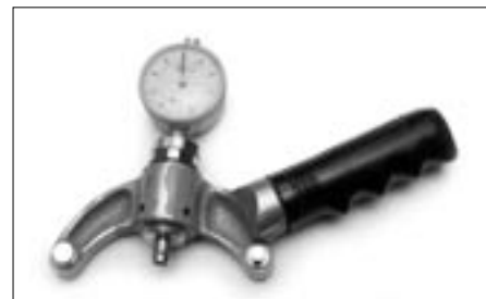
Figure 1. The Hozan Tool Industry, Inc. spoke tension meter C-737 used in this investigation
