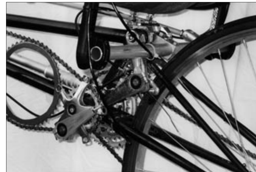
Figure 2. Close-up of the arm powered rowing/steering mechanism
